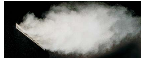
Air jet pattern of WSD above: horizontal air jet left: one jet inclined upwards and one jet downwards
