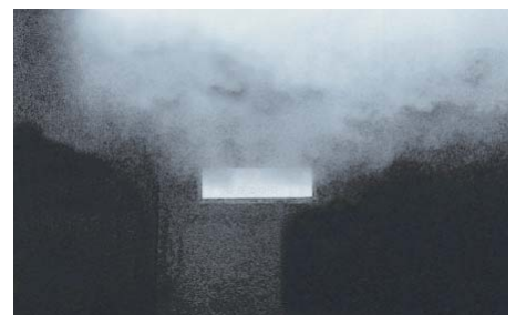
Air jet pattern of BF Asymmetrical jet direction
