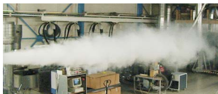
Air jet pattern of DW-V2
